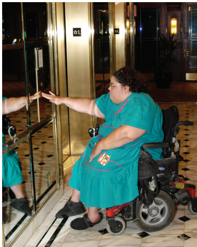
Keep obstructions like planters and trash cans away from the buttons at an elevator to ensure accessibility.
